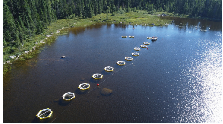
Aerial view of limnocorrals installed in the littoral zone of Lake 378 at the IISD-Experimental Lakes Area as part of the pELastic Project. Limnocorrals received additions of microplastics to simulate a gradient of plastic pollution. Photo credit: Desiree Langenfeld
