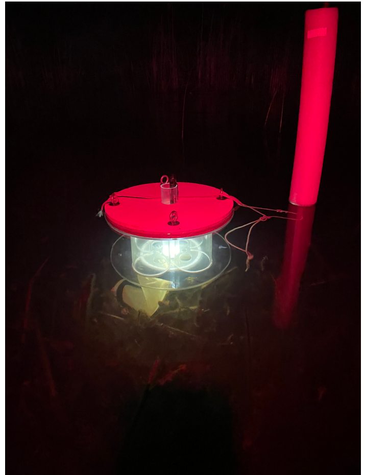
Larval light trap in situ during the night. The light causes phototaxis in larval fish which allows for sampling. Photo credit: J. Powell
