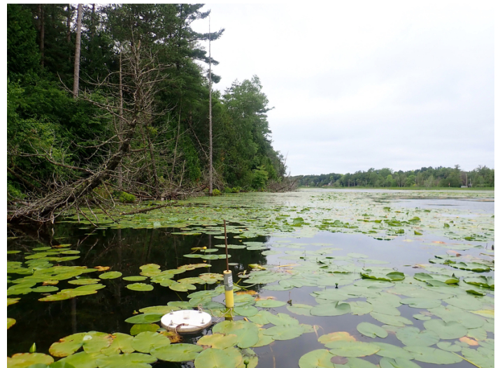
The traps are secured to a support column driven into the lake sediment. Photo credit: J. Powell
