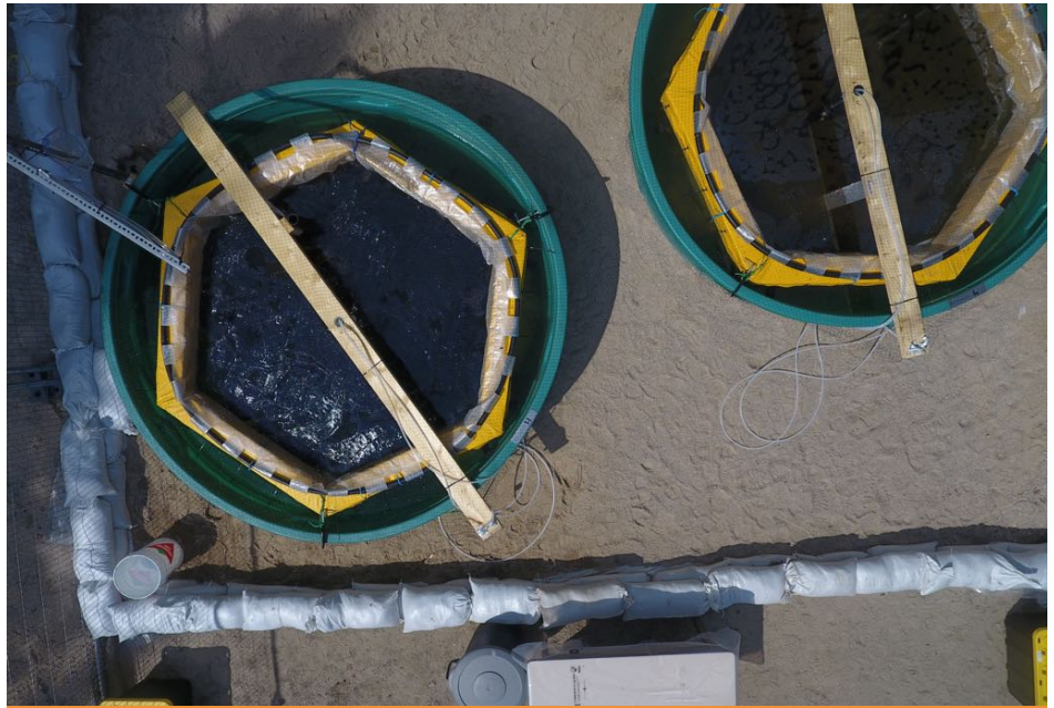
Slick, man: Shot from above via drone of the high (left) and low (right) diluted bitumen additions (photo credit: IISD-ELA)
