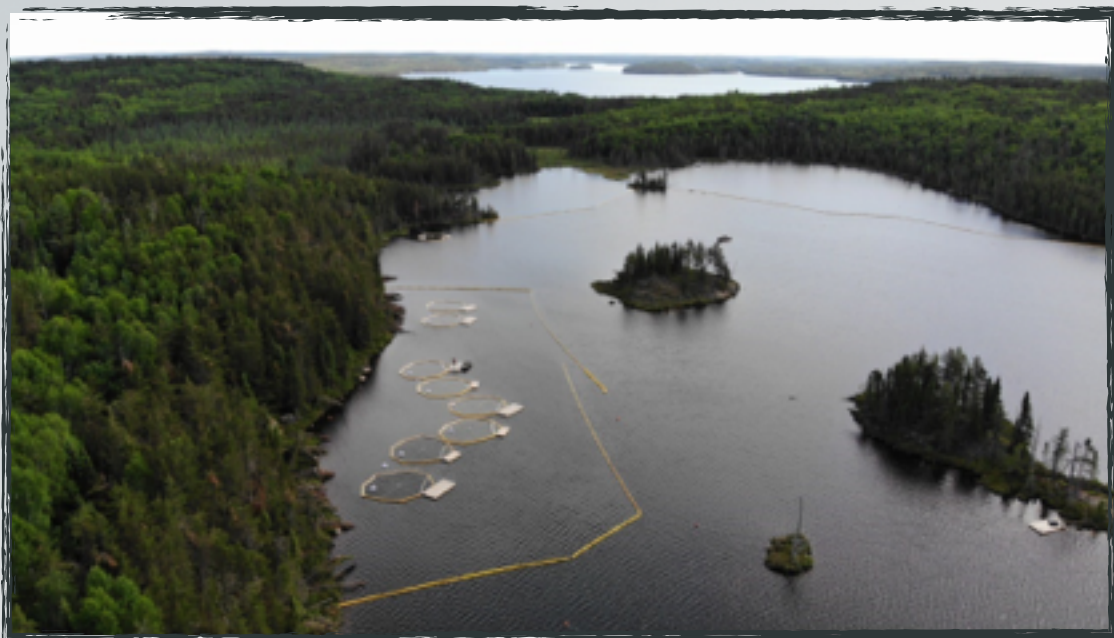
Aerial drone image of the BOREAL study to examine the environmental effects of a diluted bitumen spill on lakes. This experiment consisted of adding diluted bitumen to a series of nine large limnocorrals suspended in Lake 260 of the IISD-Experimental Lakes Area in Northwestern Ontario. Booms were set up across the lake to contain any inadvertent oil spills. Photo : Dr. Jose Rodriguez-Gil
