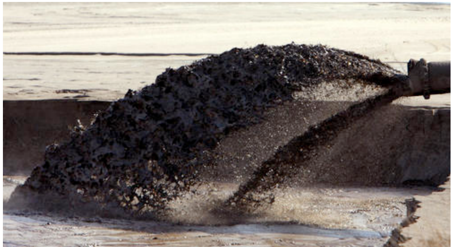
Oil sands tailings entering a holding pond near Fort McMurray, Alberta. Credit: Larry MacDougall, Canadian Press.
