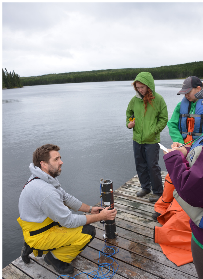
Lecture in the great outdoors: Aquatic and Experimental Limnology students learn about the proper use of a Van Dorn bottle from Instructor Mike Rennie. See story on page 8. Photo credit: Kerri Finlay.
